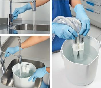
Rinse the aspiration system by sucking in 2 litres of cold water.
